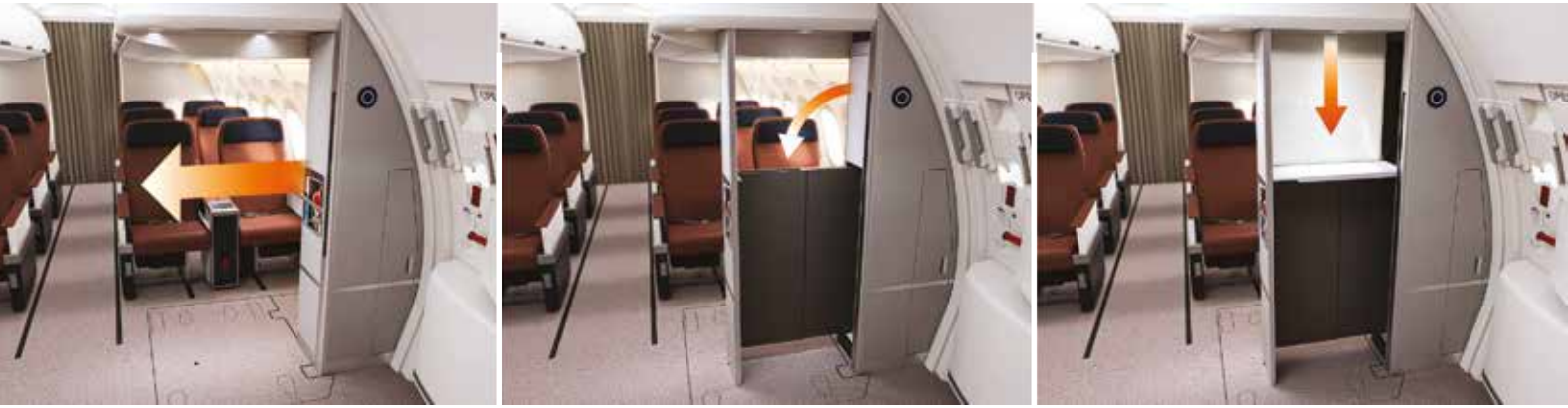
▲ Collins' Prime concept has a monument which can be stowed to allow space for a wheelchair user
