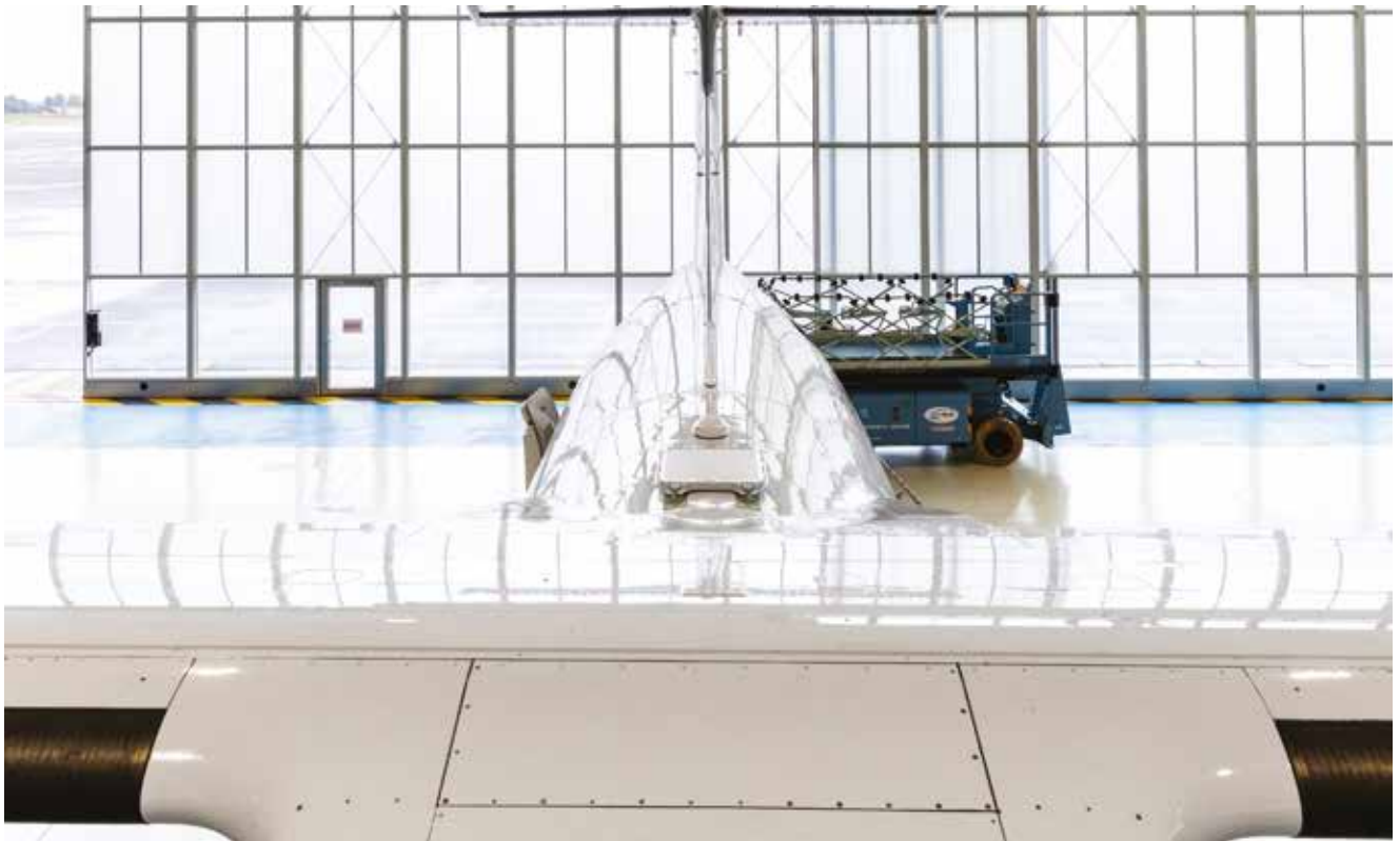
▲ Starlink aerial mounted on an ATR 72-600
