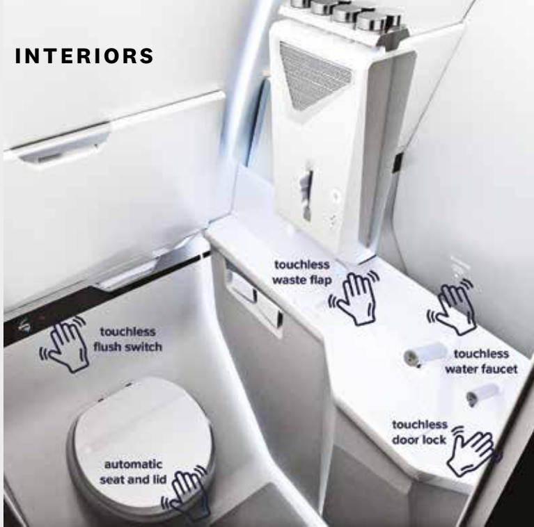
Left: Diehl Aviation is installing touch-free features in aircraft lavatories
