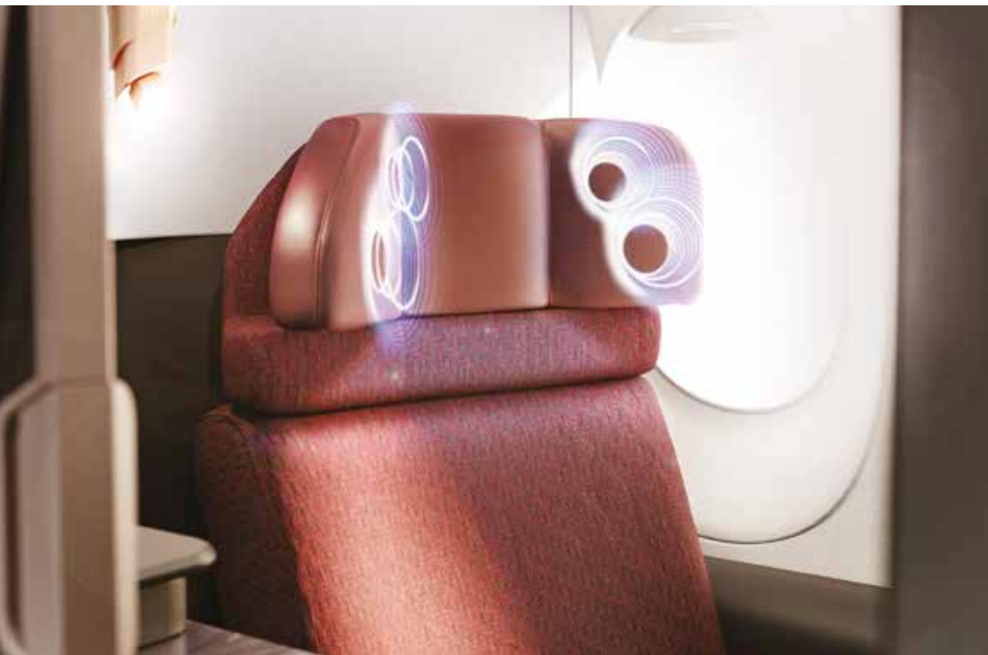
◀ Euphony provides high-quality sound to individual passengers without disturbing fellow travellers
