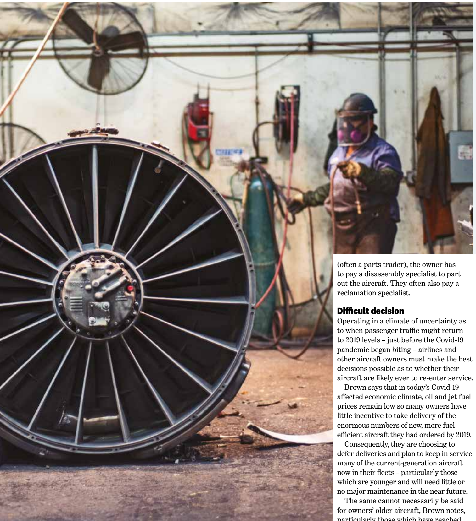
Above: Mastermelt Aero is able to recycle materials in the engine to recover the superalloys, other exotic alloys and precious metals
