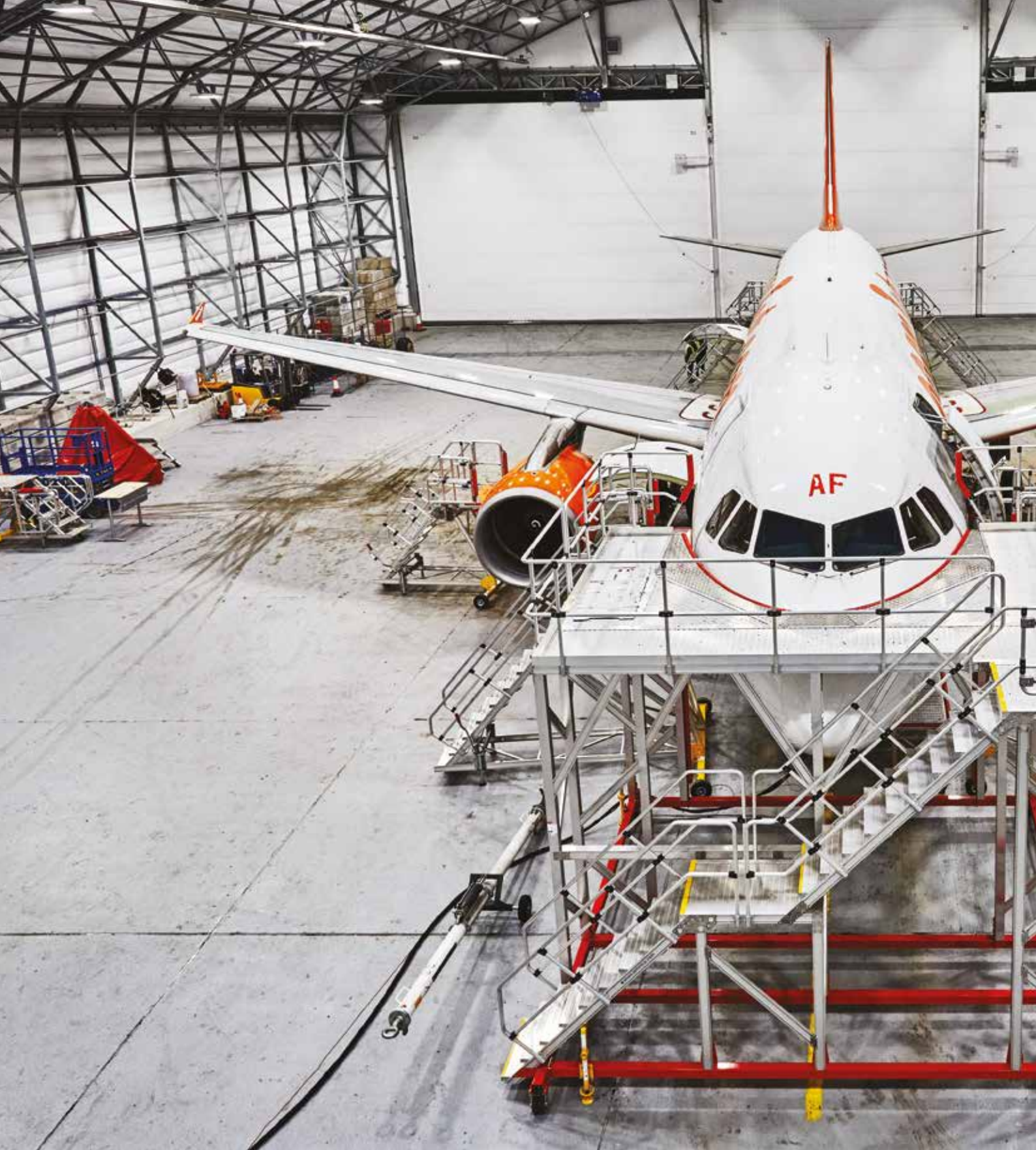
Legislation requires employers in the aviation sector to provide equipment such as access stairs and platforms. All photos: Semmco
