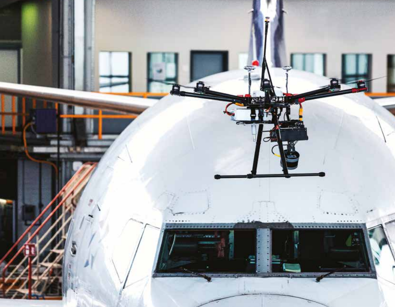
1. An AI-assisted inspection drone performs an automated visual inspection of a Boeing 737-500 at a hangar in Lufthansa Technik's base in Hamburg, Germany
