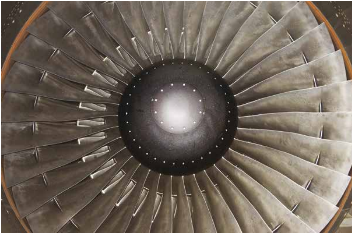
▲ General Electric CF6-80E1 turbofan engine from an Airbus A330-200
