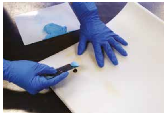
▲ For deep surface defects, the affected areas can be rebuilt using Alexit-FST EdgeFiller
