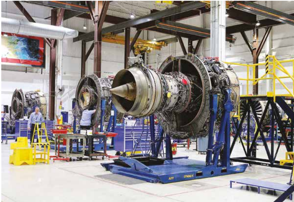
The famously reliable RB211-535 engine's modular design supports maintainability
