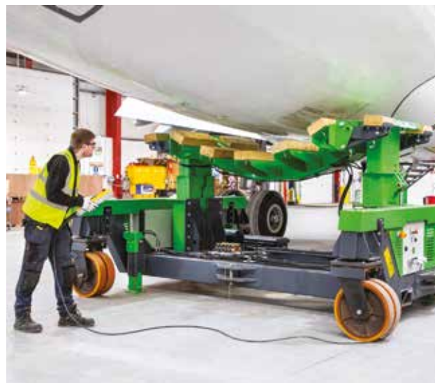
▲ EirTrade's unique jack allows landing gear to be dismantled first
