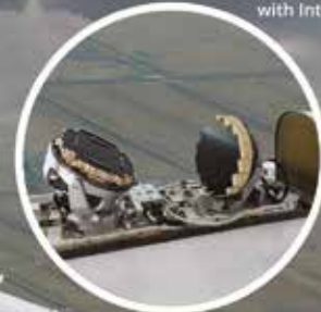
Ku-band Tail Mount Antenna with Intelsat FlexExec
