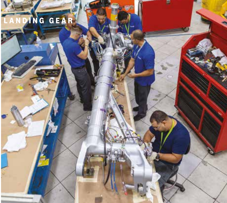
Left: Landing gears are mechanical marvels; keeping them in good working order is a complex and specialised task Below: Safran Landing Systems operates five landing gear MRO facilities of its own, including at Cheltenham in the UK. Photo by Luca Sage/CAPA Pictures/Safran
