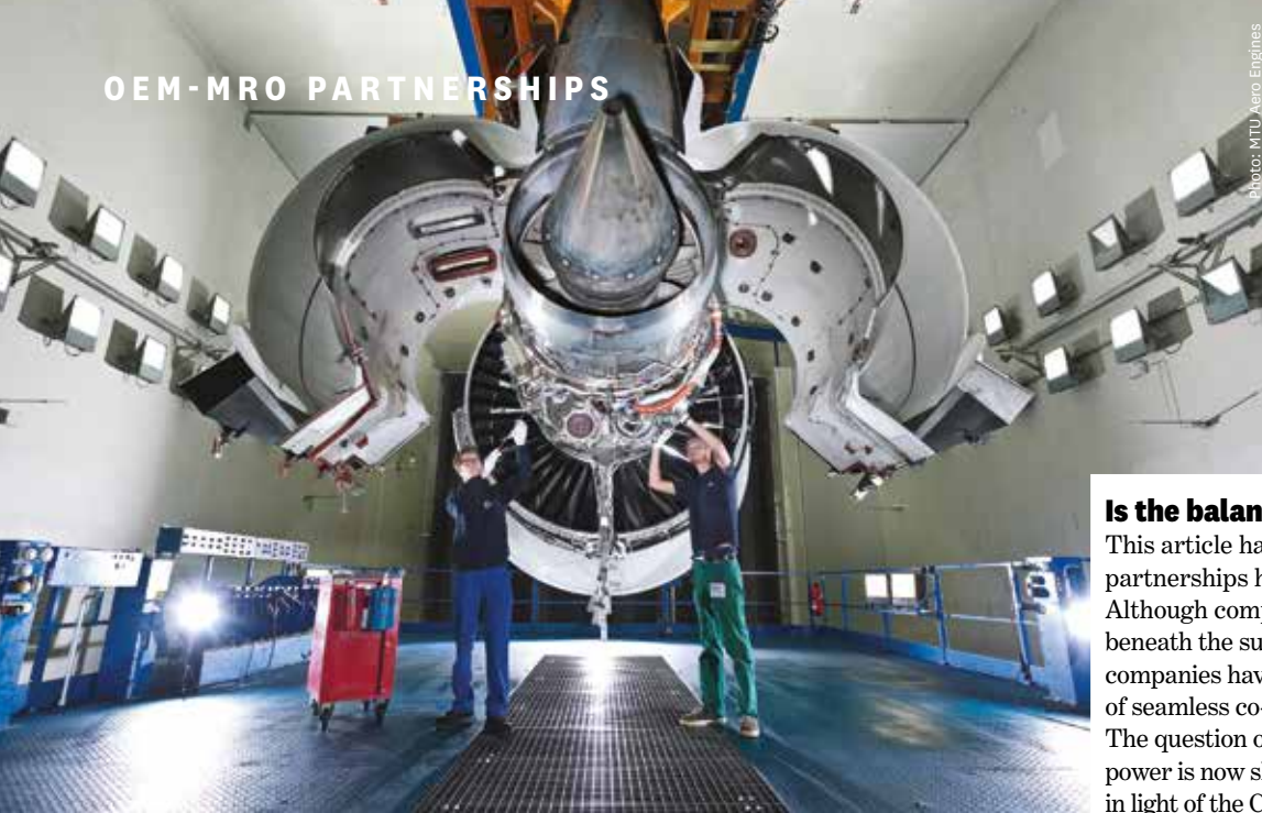
Left: Engine OEMs have a longer history of aftermarket involvement than their airframe and component counterparts. Pictured is a PW1100G-JM engine in the test cell at MTU Maintenance Hannover
