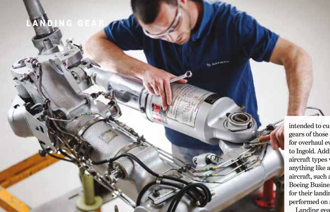
Left: A Safran engineer works on an ATR-72 main landing gear. Photo by Adrien Daste/Safran
